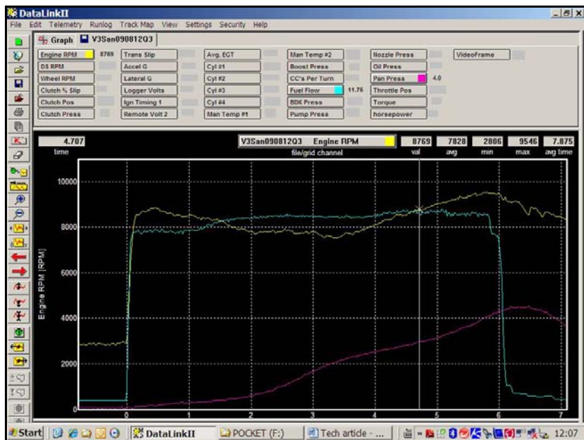
Datalogger screen shot showing engine rpm, fuel delivery to engine (GPM) & pan pressure (Psi).
